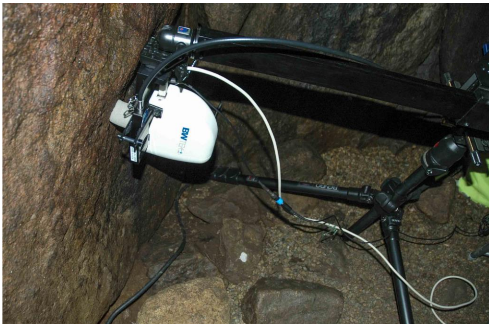
Figure S2. The portable Raman microscope BWTEK innoRam 785H in the dolmen 3, orthostat 1, of the tumulus of the Mont-Saint-Michel (Carnac, Morhiban, France).
